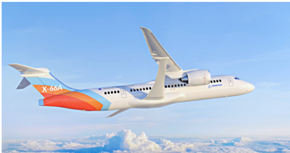
Figure 1. Transonic Truss-Braced Wing Aircraft. Source: NASA and Boeing.
