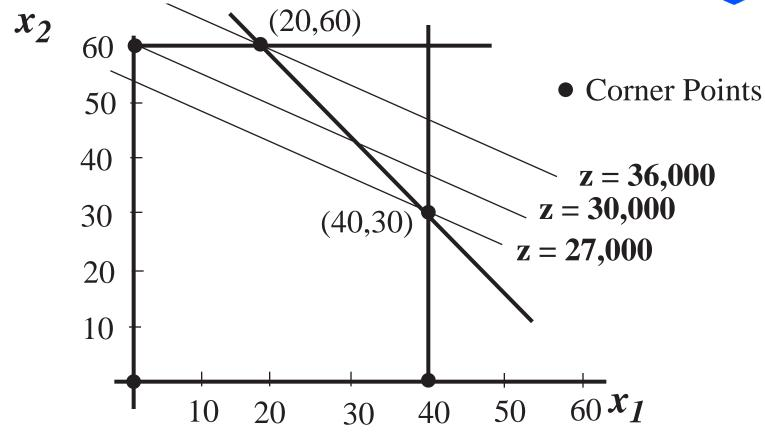
Note: Optimal Solution  $(x_1, x_2) = (20,60)$  vessels
