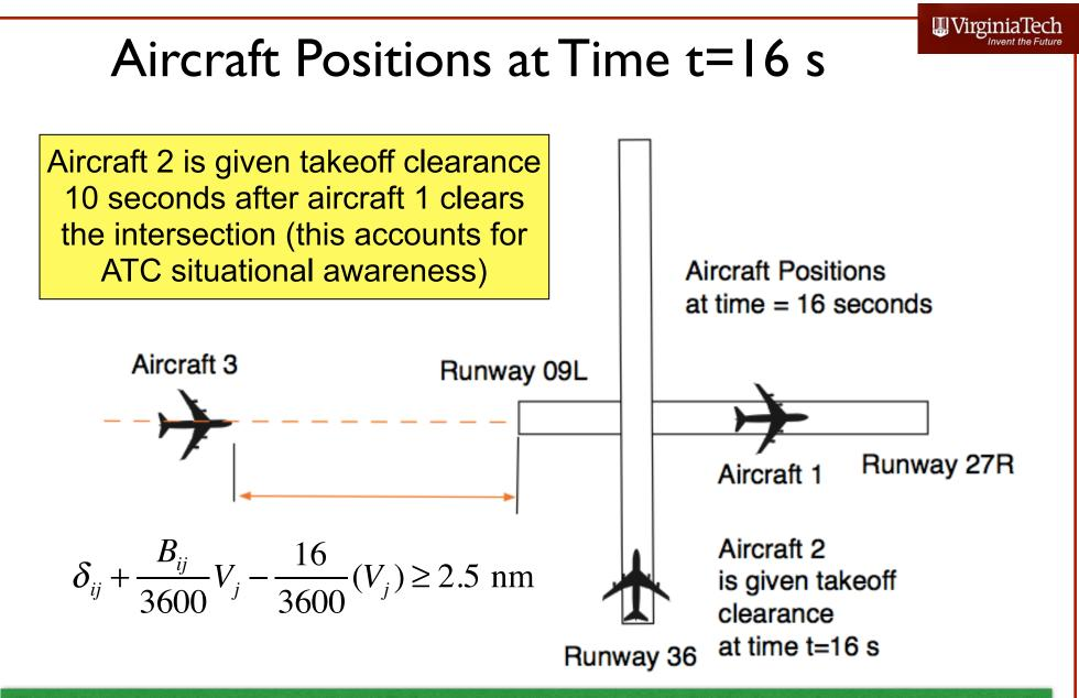
For departures on runway 36, it is desired that when the departing aircraft (aircraft 2) is cleared for takeoff, the next arrival to runway 09L (aircraft 3) be no less than 2.5 nm from the arrival threshold to 09L
