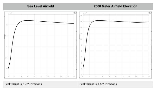
The peak thrust reduction is 27%. The density of air decreases 22% from sea level to 2,500 meters in airfield elevation.
