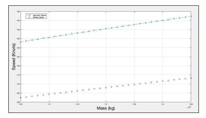
d) The large twin-engine jet aircraft (similar to the Boeing 787-8 - see Figure 4) has a maximum lift coefficient  $C_{l \max}$  of 1.85 (with flaps down 10 degrees in the takeoff configuration - see Figure 4). Find the initial safe climb speed (1.2 times the stall speed in the takeoff flap configuration) at the maximum takeoff mass of 230,000 kilograms.
