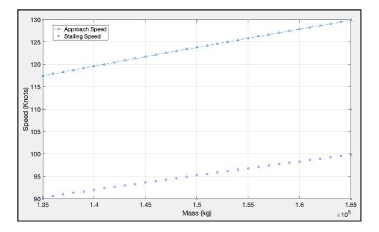
c) Find the **approach speed** for the twin-engine aircraft when the aircraft lands at Bogota International airport - Colombia - at 8360 feet above sea level conditions) at 165,000 kgs. Comment on the difference in the approach speeds at sea level and in Bogota.
