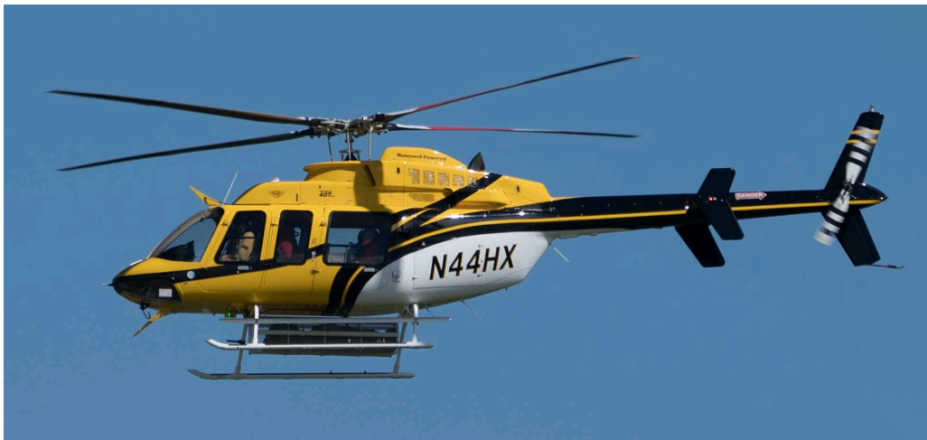
Bell 407 helicopter Single Allison 250-C47B engine (813 HP) 6,000 lbs. maximum takeoff weight
