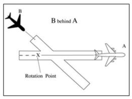
1. Aircraft landing on a crossing runway behind a departing aircraft that requires wake turbulence separation behind it if the arrival flight path will cross the takeoff path behind the departing aircraft rotation point. (See FIG 3–10–11.)
