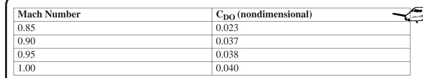
The engine manufacturer supplies you with the following data for the engines of this aircraft:
