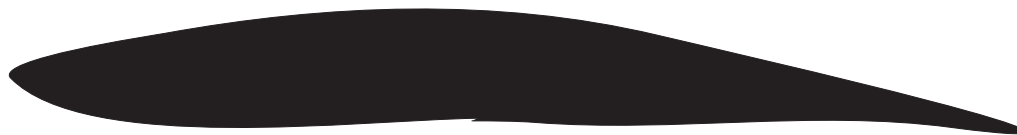
Wing cross section (cruise condition)
