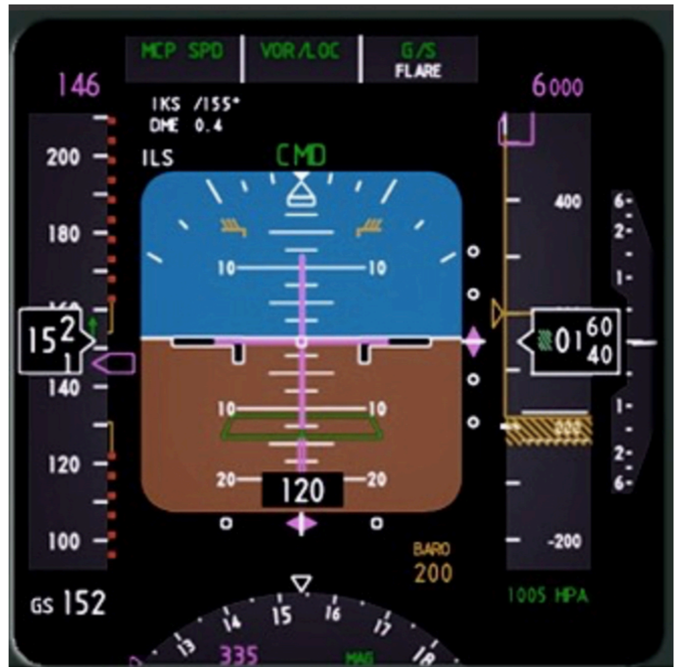
Boeing 737-800 Primary Flight Display Source: https://pmflight.co.uk/737-simulator-pfd/
