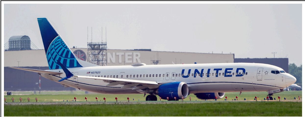
Figure 1. Aircraft Considered in the Runway Length Analysis of HPN. Picture Source: A.A. Trani. Boeing 737-9 (Max) with CFM LEAP-1B engines. Aircraft maximum design takeoff weight is 189,900 lbs. and 193 seats in a two-class layout.
