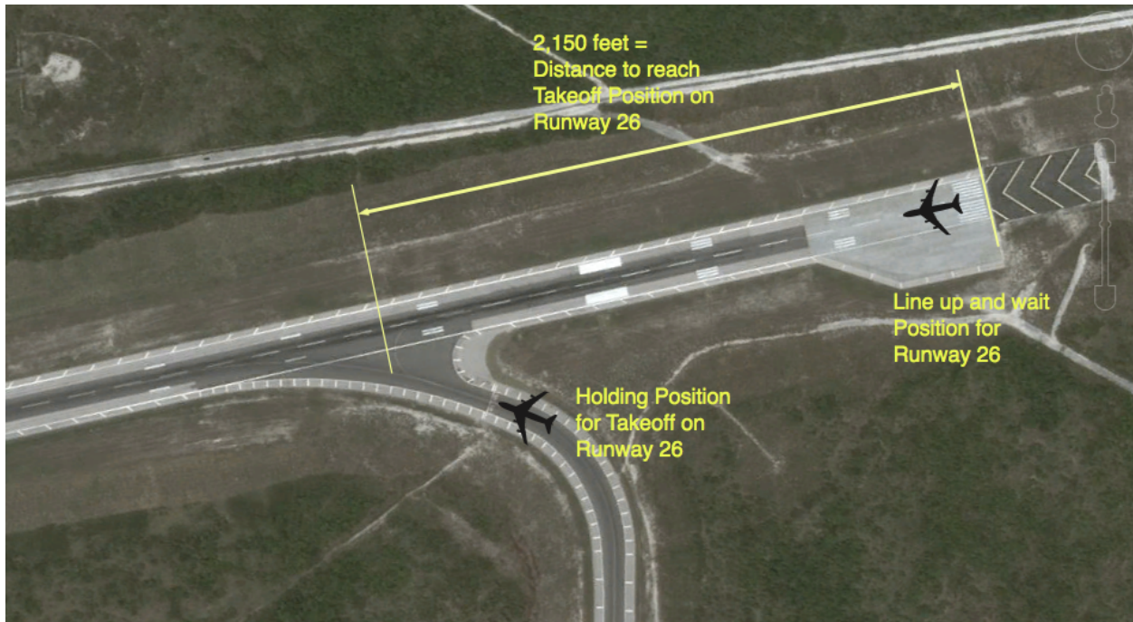
Figure 2. Punta Cana Airport Configuration for West Flow (Takeoffs and Landings on Runway 26).
