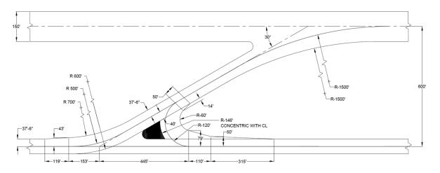
The recommended standard for high-speed runway exits is 600 feet (between runway and taxiway centerlines).
