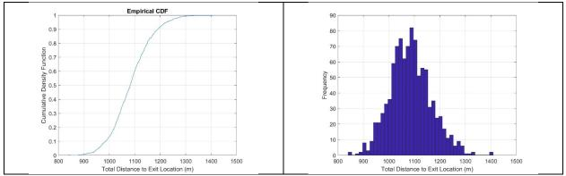
To accommodate 85% of aircraft, the exits should be located at 1850m, 1550m, 1150m for Boeing 787-8, Airbus A320, and Bombardier Q400, respectively. For bi-directional use, the locations of exits could be 1150m (Q400, B787 from opposite direction), 1500m (A320 from both directions), 1850m (B787, and Q400 from opposite direction) from each runway threshold.
