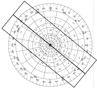
According to the analysis, 130/310 degrees of offset looks reasonable. In this case, the runway has 98.3% of wind coverage.
