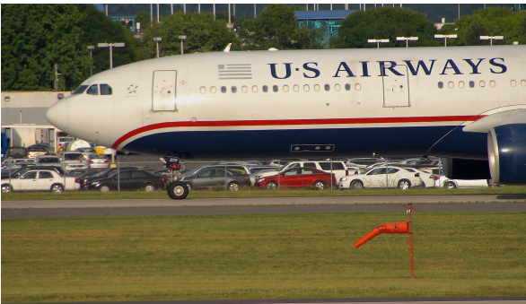
Figure 1. Airbus A330-300 Taxies to Runway 18C at CLT Airport (A. A. Trani). Note Wind Sock Located next to the Runway.
