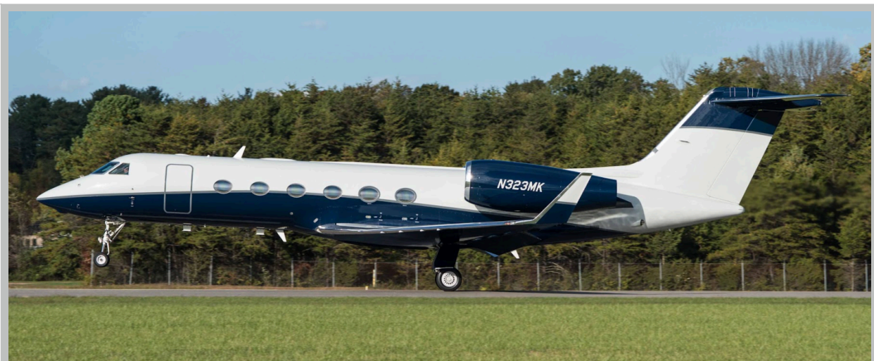
Figure 1. Gulfstream G-350 Departs Virginia Tech Montgomery Executive Airport (A.A. Trani). The G-350 is 1,500 lbs. Heavier than the G-III. The G-350 uses More Efficient Engines (Rolls-Royce Tay).
