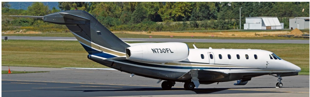
Figure 3. Cessna Citation X at BCB Airport (A.A. Trani). One of the Fastest Civilian Aircraft Flying Today (Mach 0.925 Maximum Speed).
