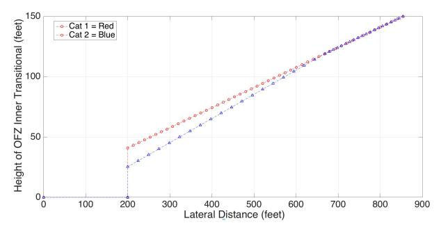
Inner Transitional OFZ surface for Airbus A350-900. Dimensions are the lateral distance from the Runway Centerline.
