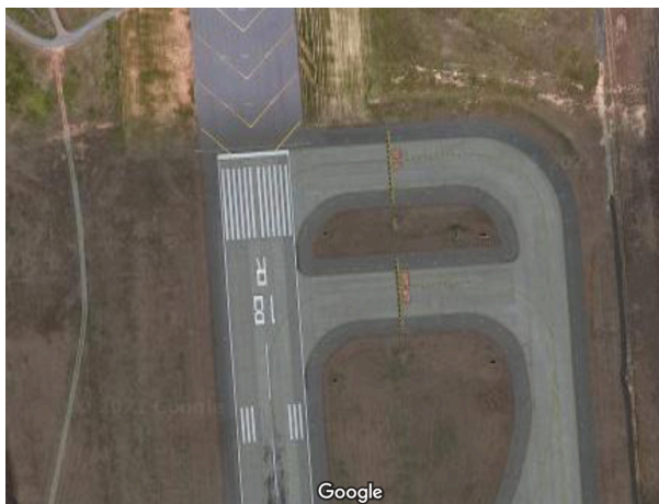
Runway 18R end at CLT airport. Note the direction of landing will be South (180 degrees from magnetic North).
