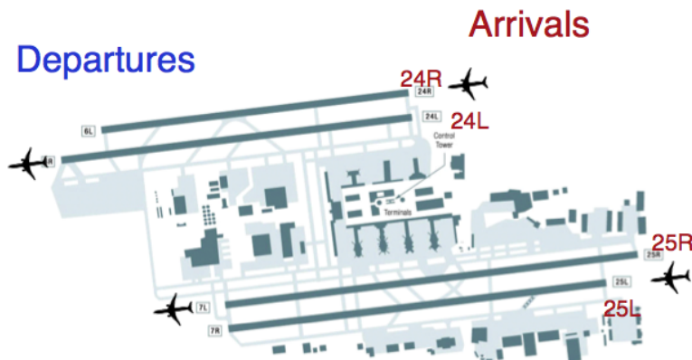
Figure 1. West-flow Operations at LAX Airport. Runways 24R and 25L used for Arrivals. Runways 25R and 24L used for Departures.
