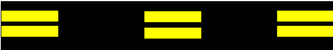
Figure B-4. Dashed Taxiway Edge Line Marking
