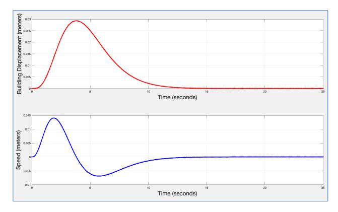
d) Select a few points to test if the gradient function is doing its job. The building horizontal speed is the derivative of the displacement as a function of time.
